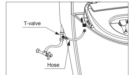
2. Existing water pipe connect T-valve.
