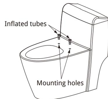
3. Place the Fixed Card on the toilet bowl where the mounting holes are. Make sure that the wash / dry gates are close to the rim and pointed down
